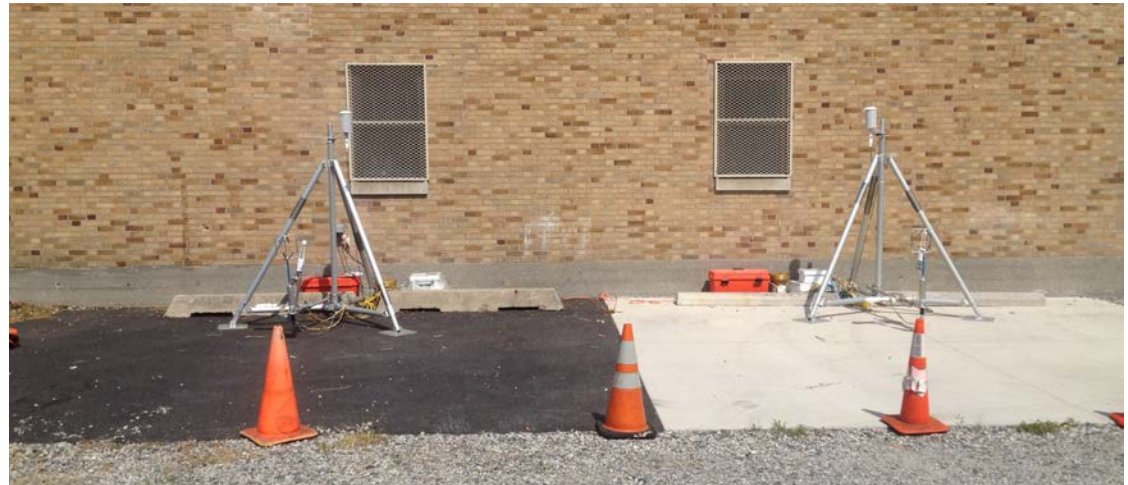
Flux towers installed at Manhattan College. Left: Asphalt. Right: Concrete.
